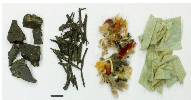
Figure 3. Different material separated from an untreated TL sample. From left to right: rubber pieces, shredded rubber, fibers, and geotextile fabric pieces. Reference line is 1 cm long.
